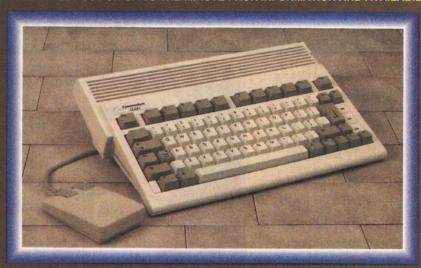
TWO MODELS: A600 FD Single 3.5" 880Kb. Floppy Drive A600 HD Single 3.5" 880Kb. Floppy Drive with Internal 20Mb. Hard Disk Drive.
