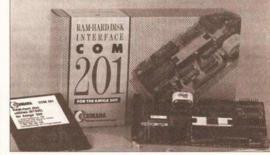
Cumana's COM-201 expansion fits into the Amiga 500's trapdoor, supplying an extra 0.5Mb of RAM, a battery backed-up clock and an ST506 hard disk controller - it's a damned fine piece of kit, and no mistake
